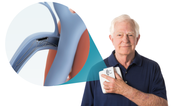
Cordella® PA Pressure Sensor System Wireless, implantable sensor for remote transmission of PA pressures
